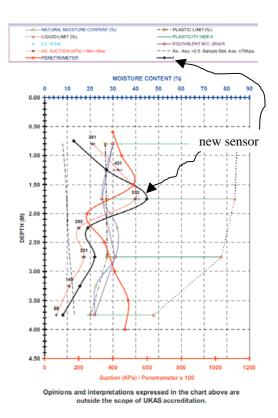
Initial results are encouraging, as we see above. All of the tests identified a zone of increased stress at around 1.75mtrs bGL.
