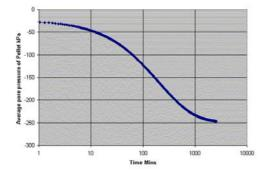
They are aiming for a 24 hour turn-around to test and deliver suction results using a new technique to cater for the difficulties we encounter at times of surge. The new test reaches equilibrium in less than 24 hours – see timeline, above.
